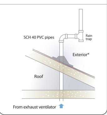
\* Please note: AAMI guidelines recommend that all EO sterilizers should be vented (exhausted) through a dedicated vent line to the outside atmosphere directly or through an emission control system. The vent should not terminate within 25 feet (7.6m) of any building air intake source or near pedestrian or animal traffic, nor should it allow EO release into or to reenter the building.
