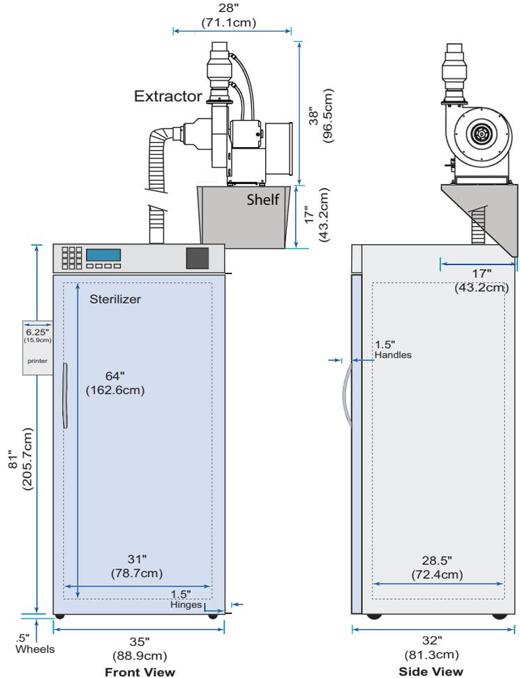
**Make Your System Zero Emissions:** The Andersen AN5200 abator is a simple, drum-based system designed to remove more than 99% exhaust stream of an EOGas 3 sterilizer. The replaceable drum employs a dry catalyst resin that converts ethylene oxide to biodegradable organic compounds. Replaceable abator drum has a 1,800 cycle capacity. Spent drums are non-hazardous.
