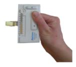
Pick up monitor and turn it upright to drain developer solution out of reading window.
