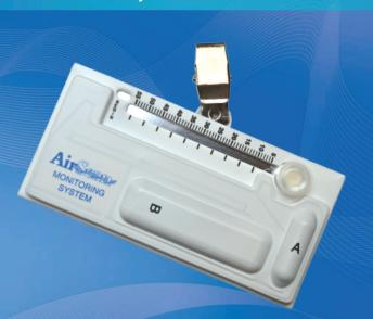
Andersen sterilisers use tiny volumes of EtO in comparison to industrial chambers, making them inherently safer. The detectors provided by Andersen routinely establish that EtO levels are below the detection limit. Both chemical and electronic detectors can do this. However, beware.... Both technologies have significant cross-sensitivities. For instance, wiping down a work bench with an alcohol based disinfectant will commonly cause both types of detector to register a positive reading.
